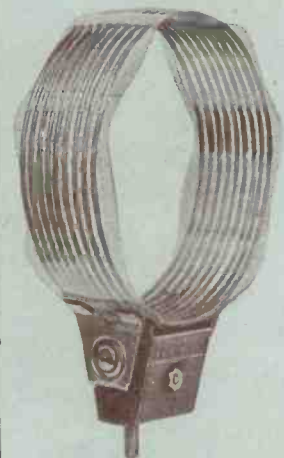
When putting a plug-in coil in or taking it out of its socket, always grip the mount and do not take hold of the coil itself
